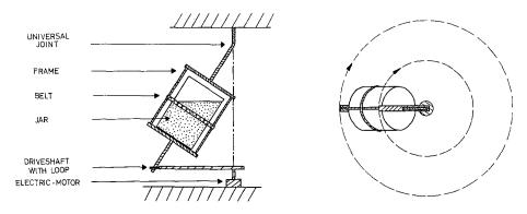
Fig. 1: Culture apparatus. Left: side view. Right: viewed from above
