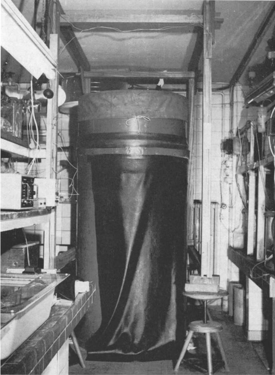
Fig. 1: Experimental arrangement of recording the directional choice. In the centre is the fibreglass reinforced polyester stand with the circular tank on top of it, on the left and right sides parts of the Helmholtz coils, on the left margin outside of the coils is a constant current source and timing apparatus for the camera
