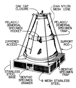
Fig. 2. Schematic of a Benthic Biotal Ocean Monitor (B-BOM). The stainless steel mesh base is 4 feet on edge and the nylon mesh cone is 6 feet tall. The device is designed to hold a variety of organisms in steel drawers, nylon pockets, and free spaces. It is effective in trapping and holding apart various indigenous species
