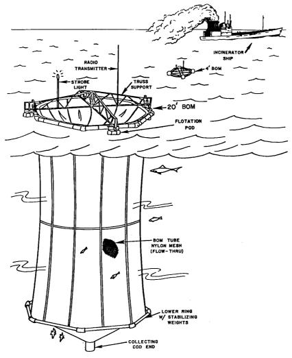
Fig. 1. Pelagic Biotal Ocean Monitors (P-BOMs) of two sizes (4 and 20 feet in diameter) deployed to monitor the incineration of toxic organochlorine residues of the manufacture of polyvinylchloride and other compounds. The BOMs, both controlled and exposed, contain a variety of organisms that are analysed after the 5–7 day exposure
