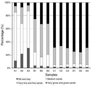
Fig. 4 Percentage of the different granulometric fractions in the sediment per sample
