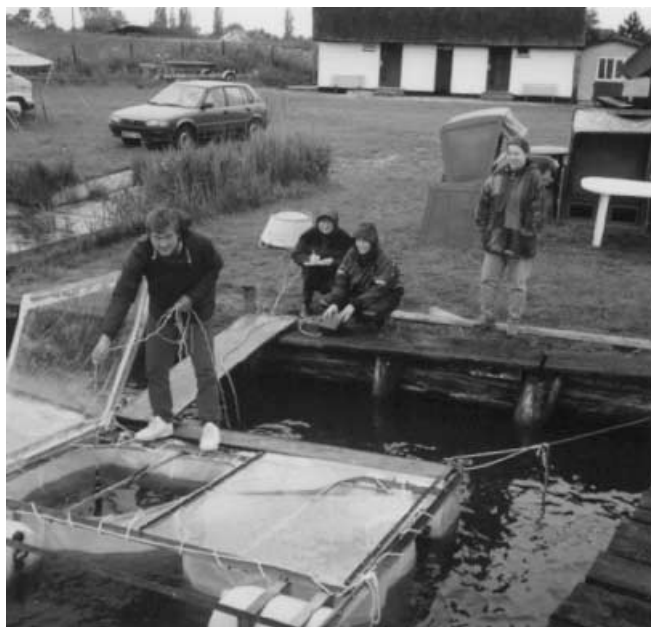
Fig. 1 Situation of 1,000-l experimental mesocosms in the Darss-Zingst estuary at the harbour of Zingst during June 1996. The Plexiglas lid of one compartment has been lifted to allow the investigator to measure the dissolved oxygen concentration in the water column
