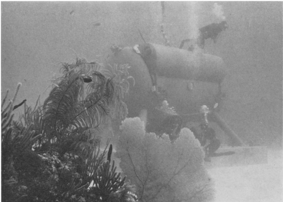
Fig. 1: Hydro-Lab, a small, one-room chamber with spartan living accommodations, rested on the sandy ocean floor adjacent to large coral heads. An unmanned life support barge was connected to the habitat by supply umbilicals
