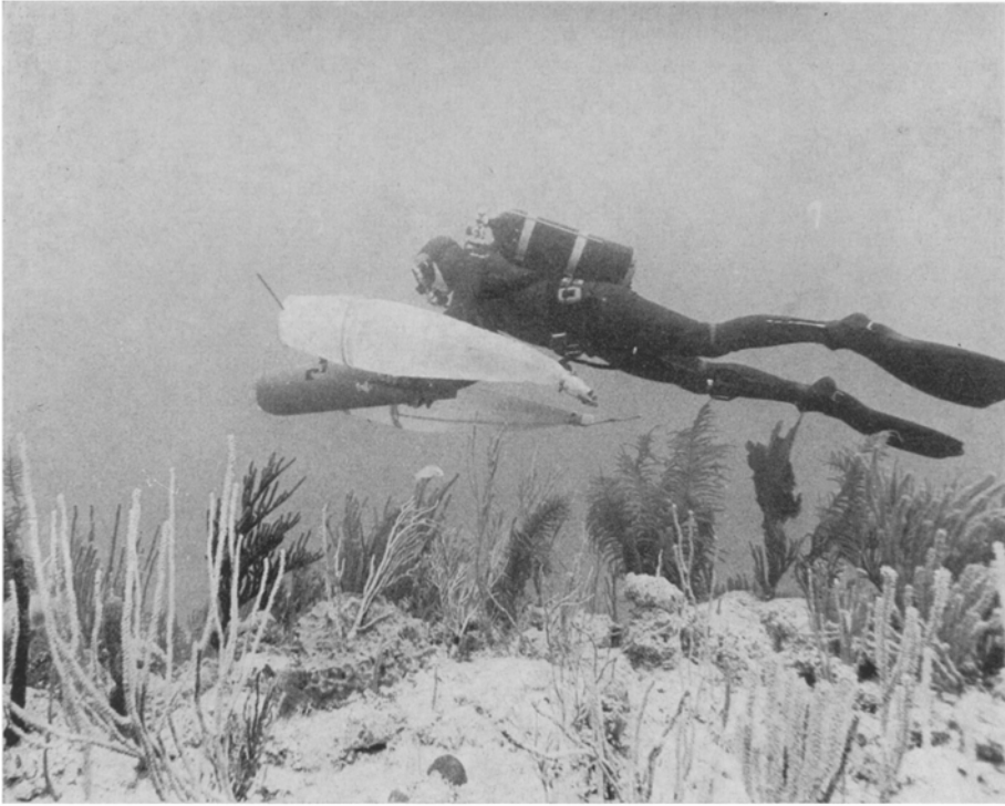
Fig. 12: Some aquanauts used diver propulsion units to reduce swimming exertion in currents and to tow sampling nets along precise routes
