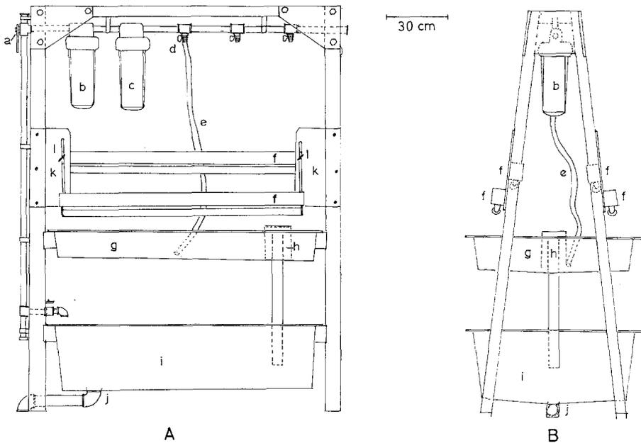
Fig. 1: Side view (A) and end view (B) of main culture tank for cultivation of *Alaria esculenta*. For detailed explanation consult text
