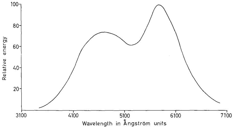
Fig. 2: Spectral distribution curve, 40 Watt daylight fluorescent lamp. (Reproduced from data supplied by Westinghouse Electric Corporation)
