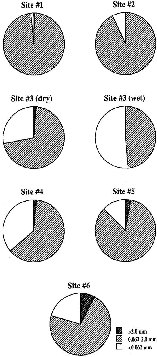
Fig. 4. Major granulometric fractions of sediments at different sampling sites (cf. Fig. 1)
